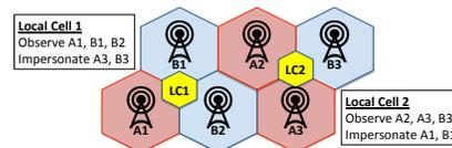
Figure 1: *NosyNeighbor* observing and impersonating commercial cellular base stations.
