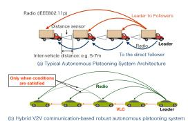
Fig. 1 VLC and Radio Hybrid Communication for Secure Autonomous Platoons
